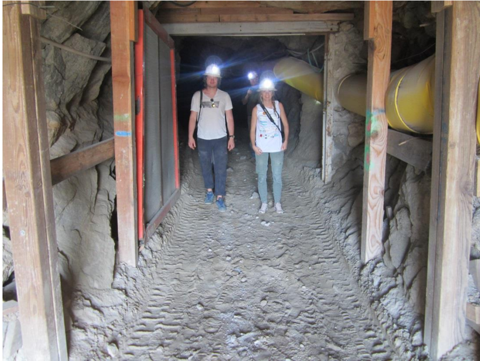
Figure 12: Students in the Gemstone mine with rather little rock support and without safety boots.
